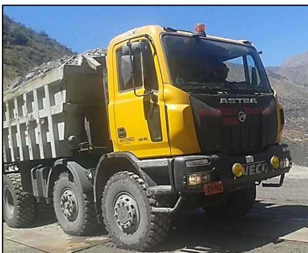
FIG.22 - "CARACTERISTICAS DE IVECO ASTRA 8X6 50 TON"
