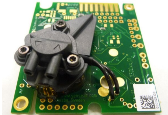
Figura 5. Sensor de CO 2 30% K-33 ICB
