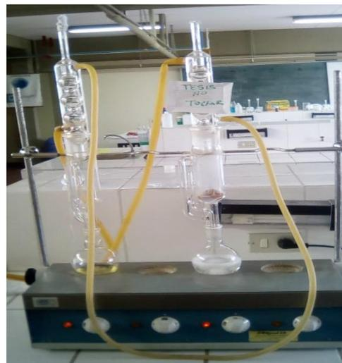
**Figura A13.30:** Extractor Soxhlet.
